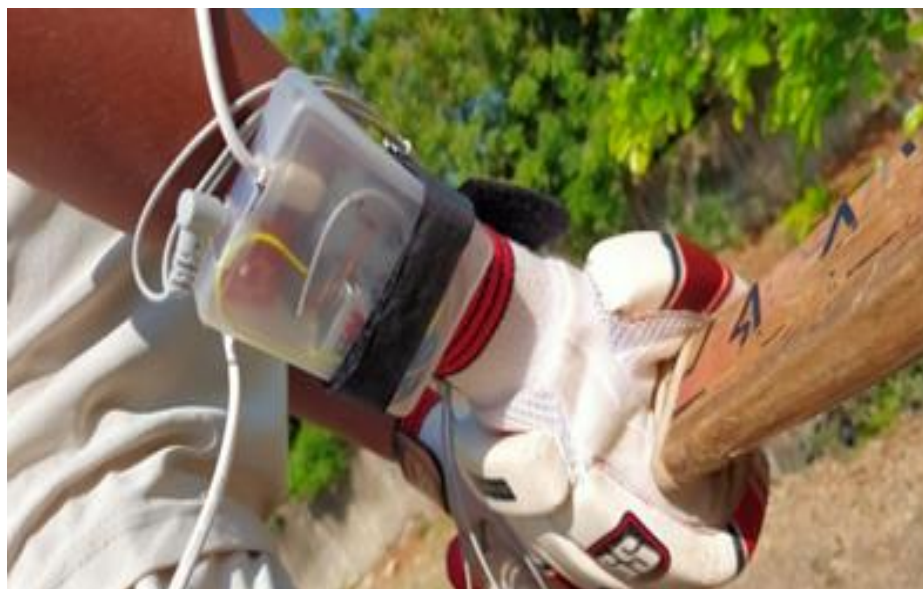
Figure 3.19 Interfacing ECG and GSR sensor module with ESP 8266
